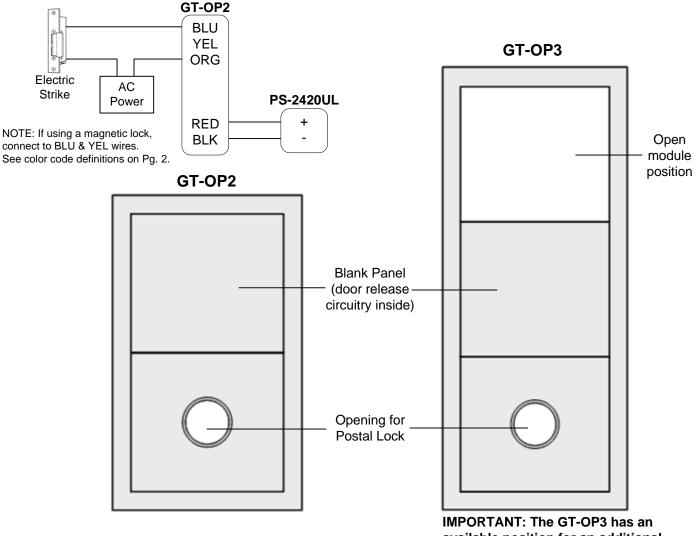
available position for an additional module. This opening can be filled by any type of module, but must be purchased separately.
